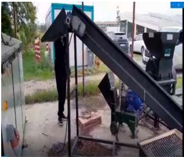
Compost machine in GTU Campus for composting waste from cafeteria and biomass (tree leaves, dried tree branches, dried weeds)
