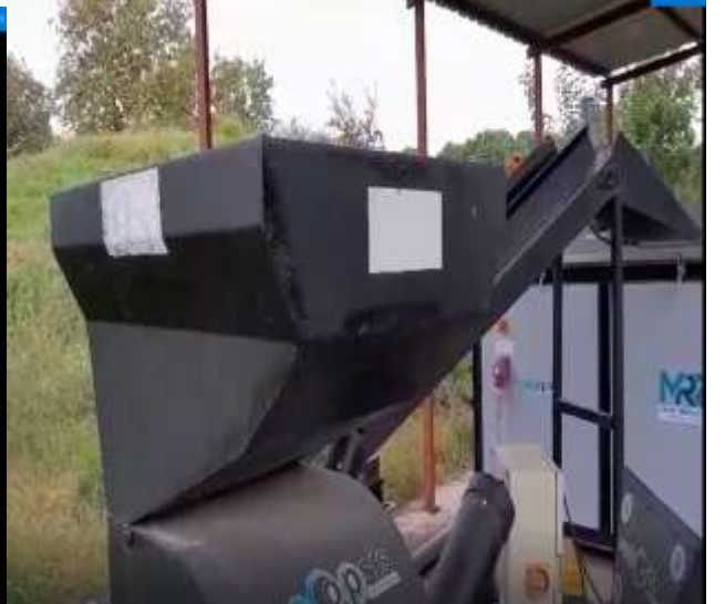
Compost machine in GTU Campus for composting waste from cafeteria and biomass (tree leaves, dried tree branches, dried weeds)
